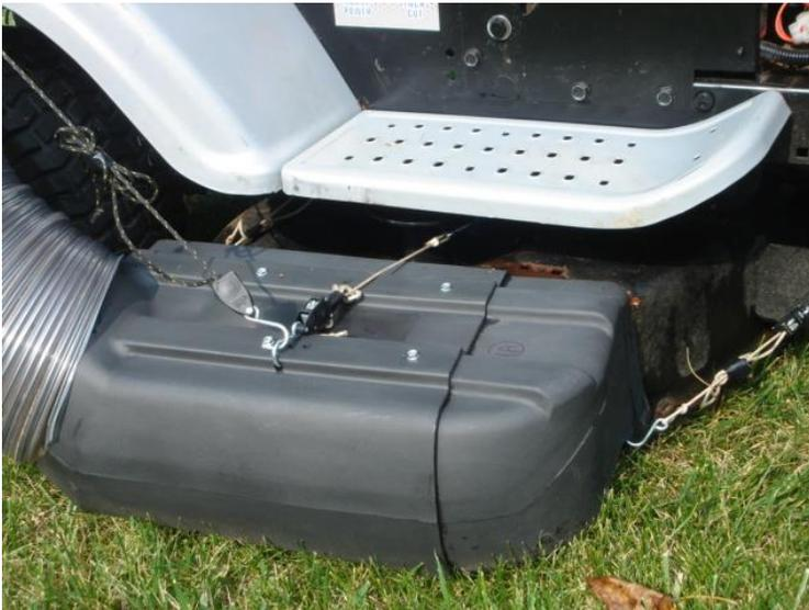
*Deck Adapter shown attached to mower deck with Discharge Tube attached. This photo shows the Deck Adapter in the proper position for use. Note the rope from the Deck Adapter up along tube that attaches to Vent Disk.*
